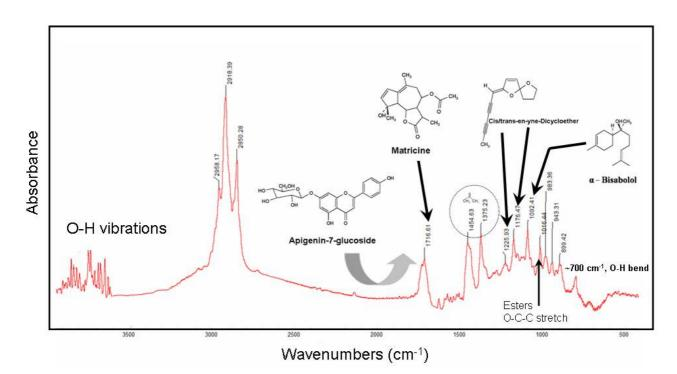
Fig. 4. FTIR spectrum of *M. recutita* L. obtained by water distillation method utilizing a Clevenger apparatus. In the insert are indicated the peak assignments of the main components along with their chemical structures as identified in the IR spectrum
