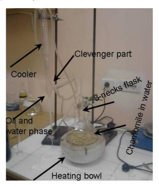
Fig. 2. Photo of Clevenger apparatus used for the extraction with steam distillation indicating by arrows the main parts.
